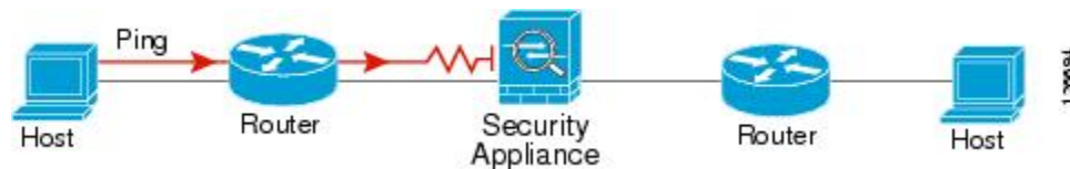
Figure 70: Ping Failure Because the ASA is Not Translating Addresses
