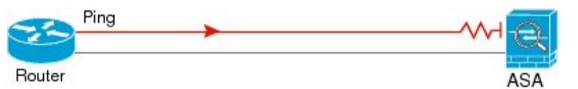
Figure 69: Ping Failure Because the ASA Has No Return Route
