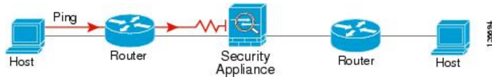
Figure 104: Ping Failure Because the ASA is Not Translating Addresses
