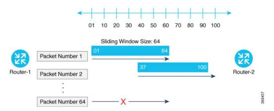
By default, the sliding window is set to 512 packets. It can be set to any value between 64 and 4096 that is a power of 2 (that is, 64, 128, 256, 512, 1024, 2048, or 4096). To modify the anti-replay window size, use the **replay-window** command, specifying the size of the window:
