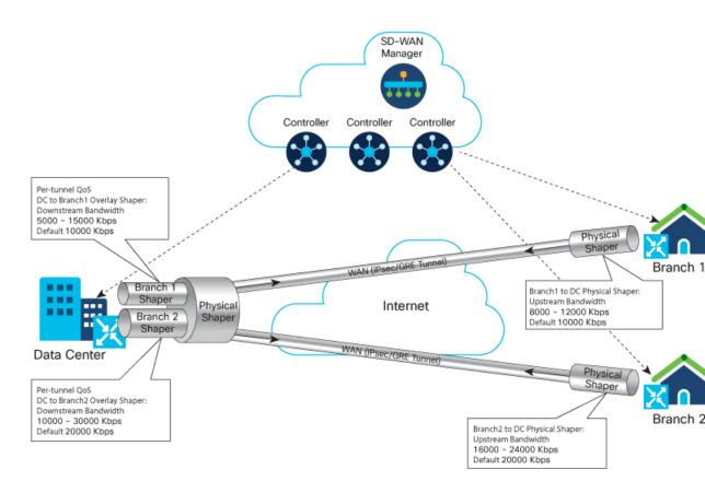
In the image, adaptive per-tunnel QoS is configured on the WAN interfaces of the spoke devices (Branch 1 and Branch 2) through Cisco SD-WAN Manager with the following configurations:
