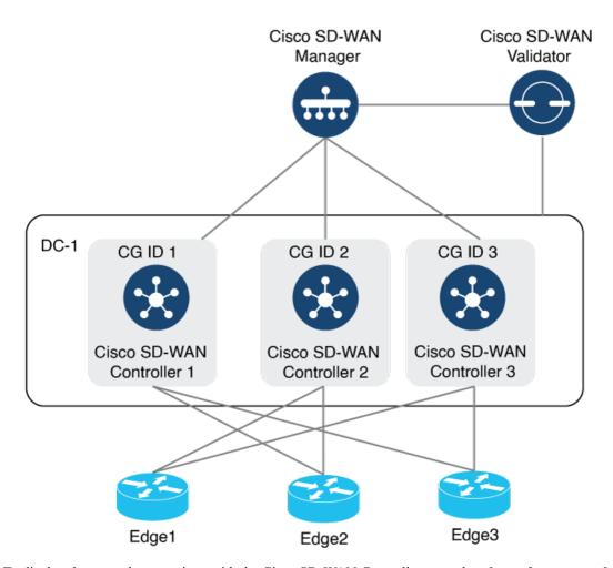
To display the control connections with the Cisco SD-WAN Controllers, use the **show sdwan control connections** command. The last column on the output, **Controller Group ID**, lists the Cisco SD-WAN Controller group that a router is in.
