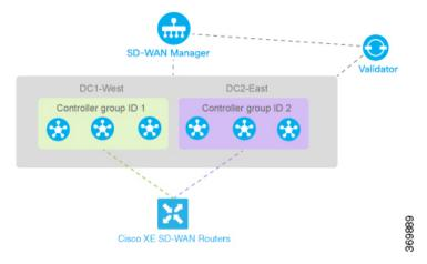
On the Cisco IOS XE Catalyst SD-WAN device router, define the controller group list and configure the maximum number of OMP sessions to be 2:
