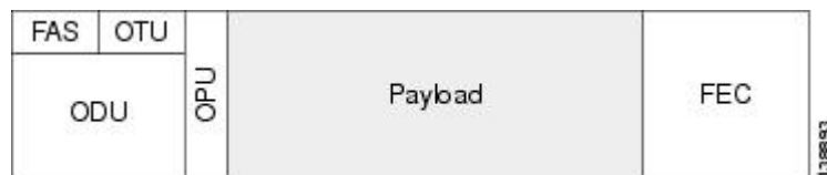
Figure 1: OTN Optical Channel Structure
