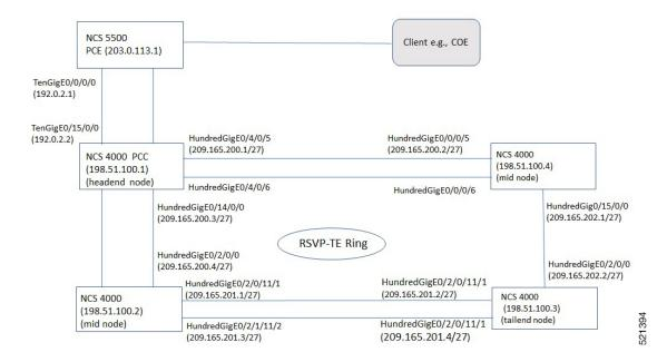
The topology has four NCS 4000 nodes for redundancy and one NCS 5500 node (PCE). The headend node (198.51.100.1) is connected to PCE (203.0.113.1) through the interface. Perform the following steps to create an RSVP-TE tunnel between the headend node (198.51.100.1) and the tailend node (198.51.100.3).
