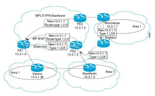
Because the sham-link is seen as an intra-area link between PE routers, an OSPF adjacency is created and database exchange (for the particular OSPF process) occurs across the link. The PE router can then flood LSAs between sites from across the MPLS VPN backbone. As a result, the desired intra-area connectivity is created.
