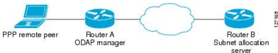
Figure 2: Subnet Allocation Server Topology
