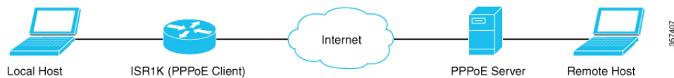
Figure 2: Sample Topology of a PPPoE Client and Server over a VLAN Interface
