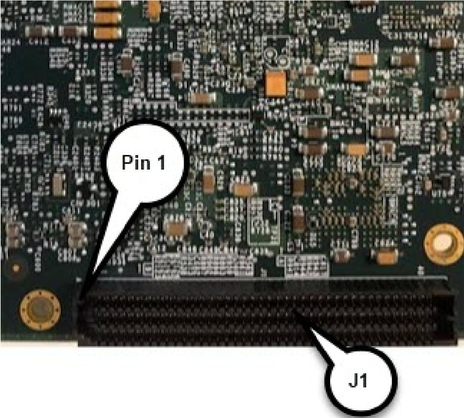
The following table lists the mating connector (SEAM lead style) options that are available to achieve specific stacking heights when coupled with the ESR (-05.0 SEAF lead style).
