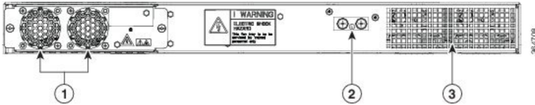
Figure 3: Rear View of Cisco ASR-920-12SZ-IM Router
