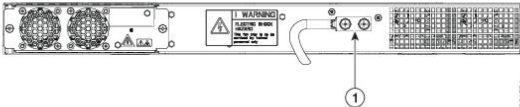
Figure 9: Attaching a Grounding Lug to the Rear of the Router
