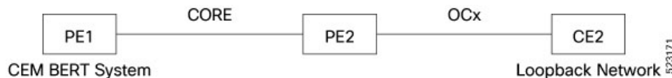
Figure 5: Configuring System CESoP NxDS0 BERT with System Direction and Speed on PE1 and Loopback as Network on CE2
