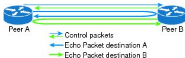
Figure 19: BFD Asynchronous Mode With Echo Packets
