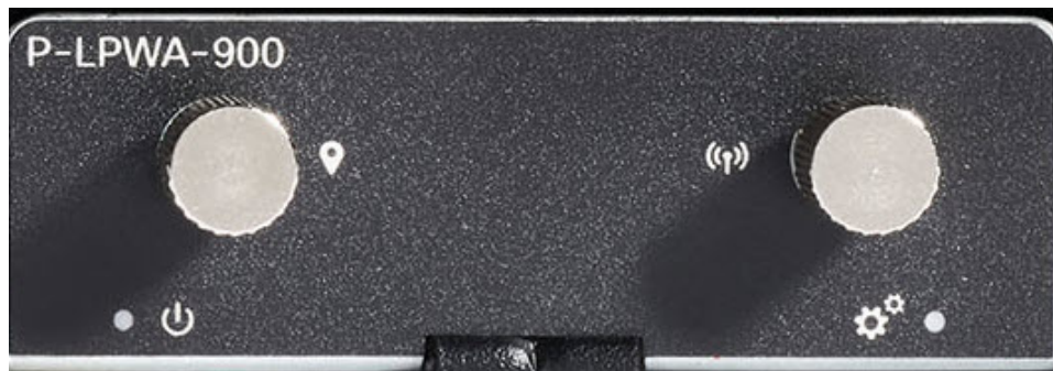
Figure 1: P-LPWA-900 LoRaWAN Pluggable Interface Module
