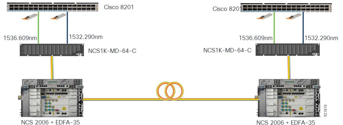
Figure 9: 400G-ZR P2P Short Haul Applications with Cisco NCS 2006
