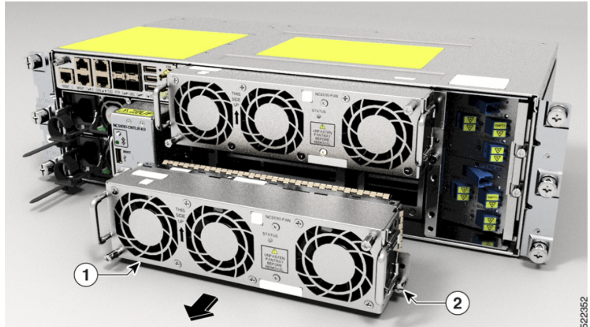
Figure 84: Removing the Fan Tray
