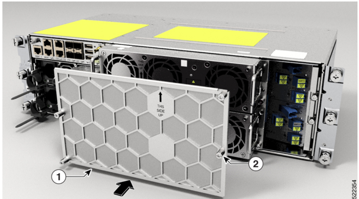
Figure 76: Installing the Fan Filter
