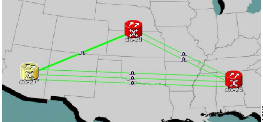
Figure 18-26 Network View with Local Link Consolidation
