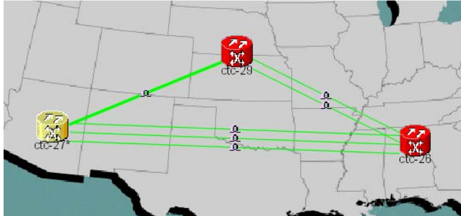
Figure 21-15 Network View with Local Link Consolidation
