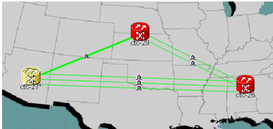
Figure 21-15 Network View with Local Link Consolidation
