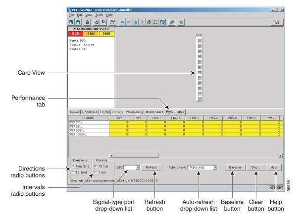
Figure 9-1 Viewing Electrical Card Performance Monitoring Information
