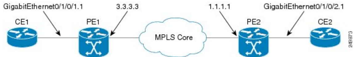
Figure 1: VPLS with BGP autodiscovery and BGP signaling
