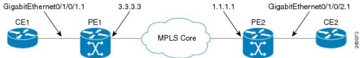
Figure 13: VPLS with BGP autodiscovery and BGP signaling
