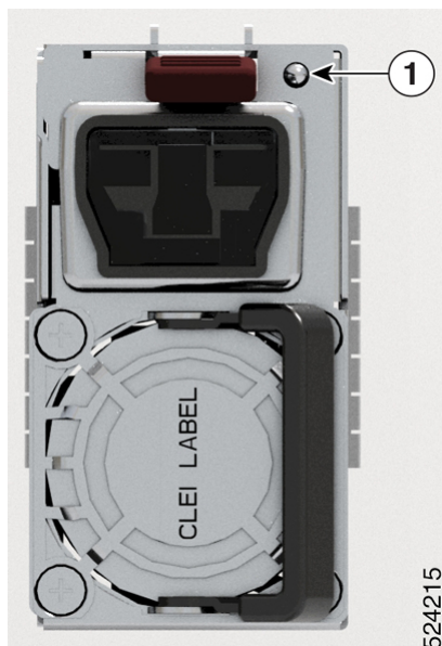
Figure 117: Power Supply LED - 8212-48FH-M Chassis
