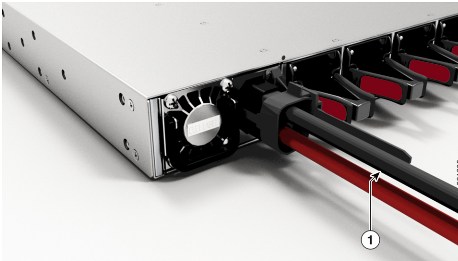
Figure 60: Connecting DC Power - Cisco 8201-32FH Router
