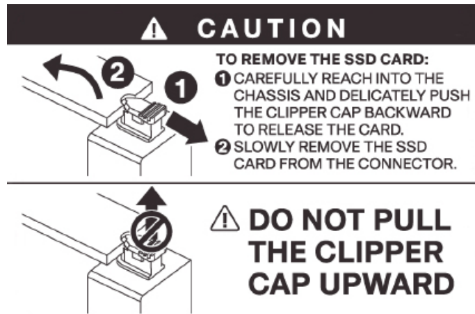
Figure 12: SSD Card Removal Instructions
