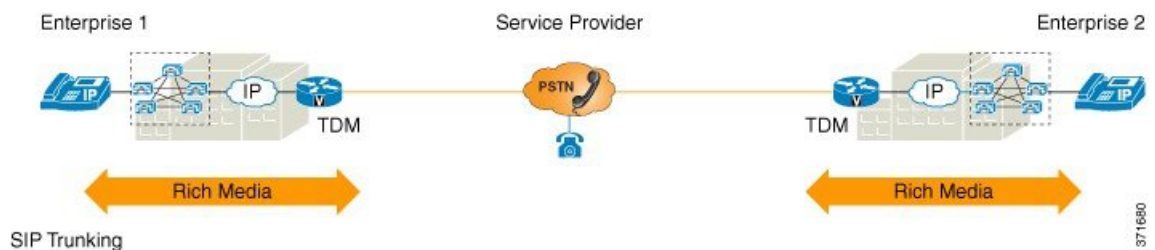
Figure 4: SIP Trunking Overcomes TDM Barriers
