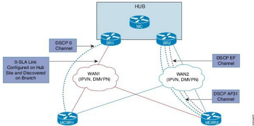
In the above illustration, the branch and hub sites are connected with red and blue ISP links. On the red ISP link, Zero SLA is configured at the hub site. Traffic exists on DSCP-0, DSCP AF31, and DSCP-EF channels on both ISP links, but on the red link probing is sent only on the DSCP-0 channel. A probe sent during the WAN discovery signals if a link is a Zero SLA link or a normal link.
