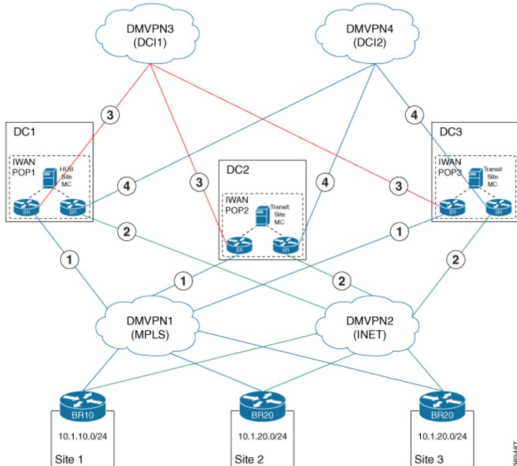
The PfRv3 Inter-DC Optimization feature can be enabled with the **inter-dc** command in domain master controller advanced mode. All hubs in the network must be connected through WAN overlay or DCI overlay. All hub and transit hub masters must be enabled with this feature locally. WAN overlay is configured by defining a WAN interface using the **domain path** command. DCI overlay is configured by defining a DCI interface using the **domain dci-path** command.
