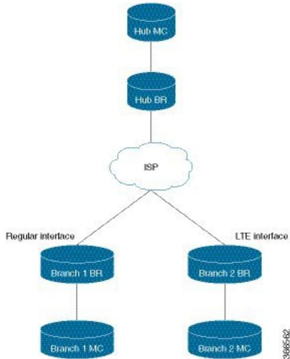
A hub branch router communicates to two branch routers Branch 1 Router and Branch 2 Router via ISP. Branch 1 Router has a regular interface, while Branch 2 Router has an Long-Term Evolution (LTE) interface. The LTE interface requires different probing parameters on the channel connected to the interface as LTE radio channels are established when data needs to be transmitted over the interface and radio frequency band occupies the transmission.
