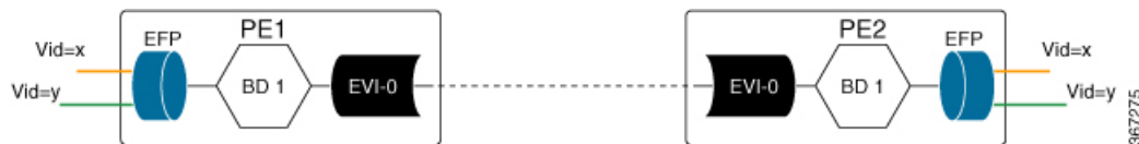
Figure 2: VLAN Bundle Service Interface
