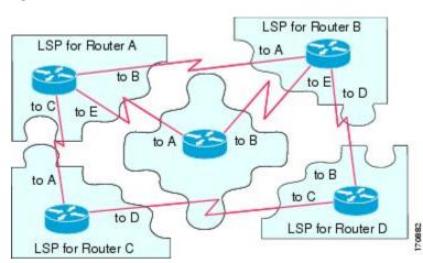
The figure below shows each router in the IS-IS network with its fully updated link-state database, after the adjacencies have been formed among the neighbor routers.
