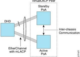
The PoAs forming a virtual LACP peer, from the perspective of the DHD, are defined as members of a redundancy group. For the PoAs in a redundancy group to appear as a single device to the DHD, the states between them must be synchronized through the Interchassis Communication Protocol (ICCP), which provides a control-only interchassis communication channel (ICC).
