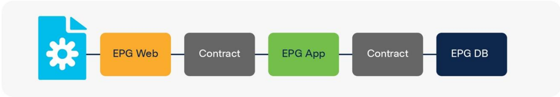
Figure 3. Cisco ACI EPG-Based Network Model
