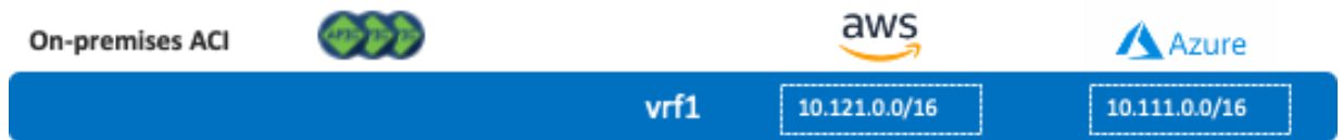
Figure 30. VRF Is Stretched Across Multiple Sites Without a Bridge Domain on the On-Premises ACI Site
