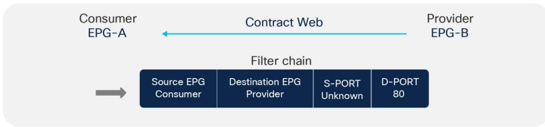
Figure 67 The Filter Chain of a contract is defined in the consumer-to-provider direction
