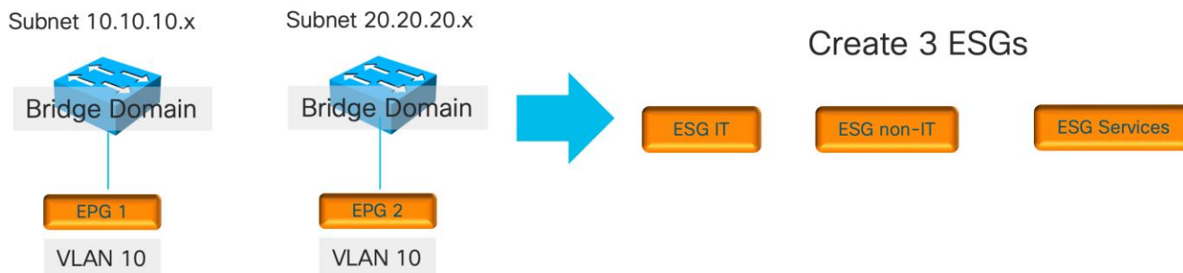
Figure 48 Using ESGs to segment the endpoints
