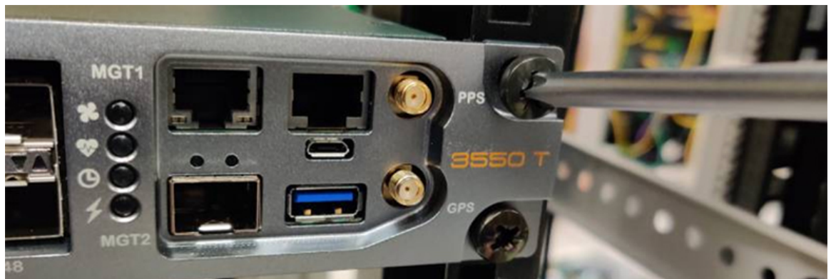
Figure 9: Fasten the Nexus 3550-T in the normal manner.
