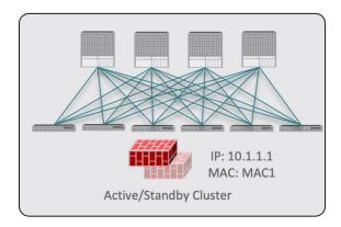
In this case, you need to provide a single PBR destination IP address identifying the active firewall node and also include information about every node in the cluster.
