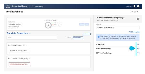
• **BFD Settings** – specifies BFD parameters for BFD sessions established between devices on interfaces that are directly connected.
