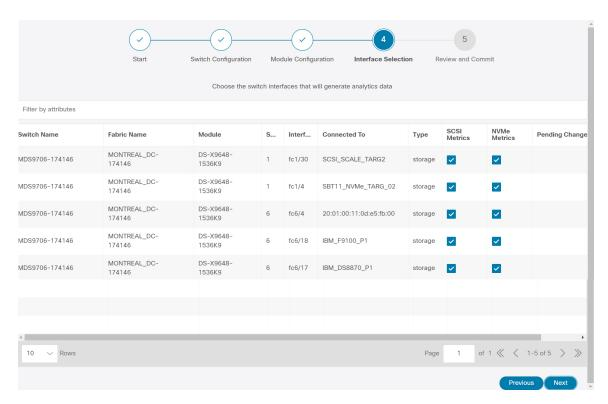
For each interface, you can enable or disable metrics. Choose check box in SCSI Metrics and NVMe Metrics column to enable or disable analytics on the desired port.
