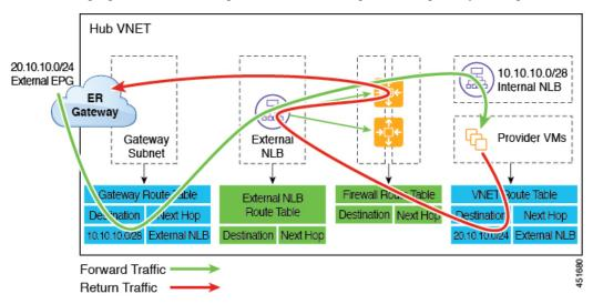
The following figure shows an example of a redirect for express route gateway to the provider EPG in the spoke VNet.
