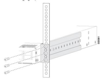
d) Tighten the 10-32 screws to 20 in-lb (2.26 N·m) or tighten the 12-24 screws to 30 in-lb (3.39 N·m).
