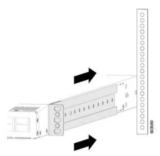
b) Gently slide the switch all the way into the rack until the front rack-mount brackets come in contact with the cabinet posts.
