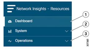
**1** Dashboard: The main dashboard for the Cisco NIR application providing immediate access to anomalies.
