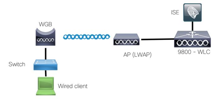
In this example, the IW3702 Autonomous Access Point (AP) is configured as a WGB and connects to the Lightweight Access Point network. Use this SSID, dot1xssiD-R, for the connection to the WLAN and use the PEAP for the authentication of the WGB to the network.
