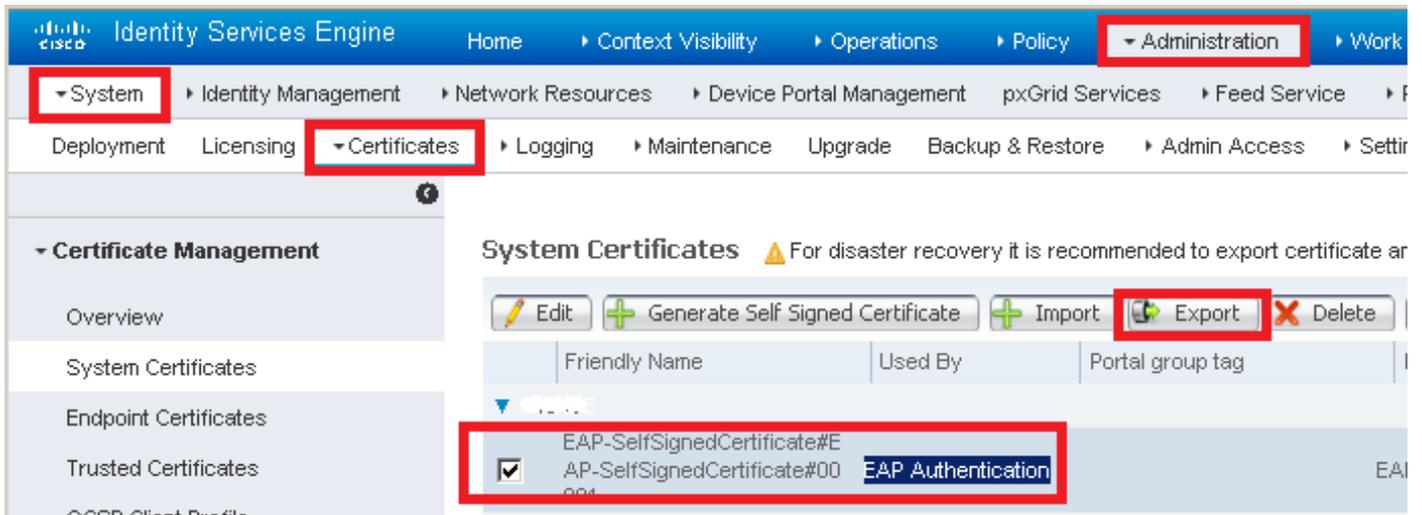
Save the certificate in the needed location. This certificate is installed on the Windows machine.
