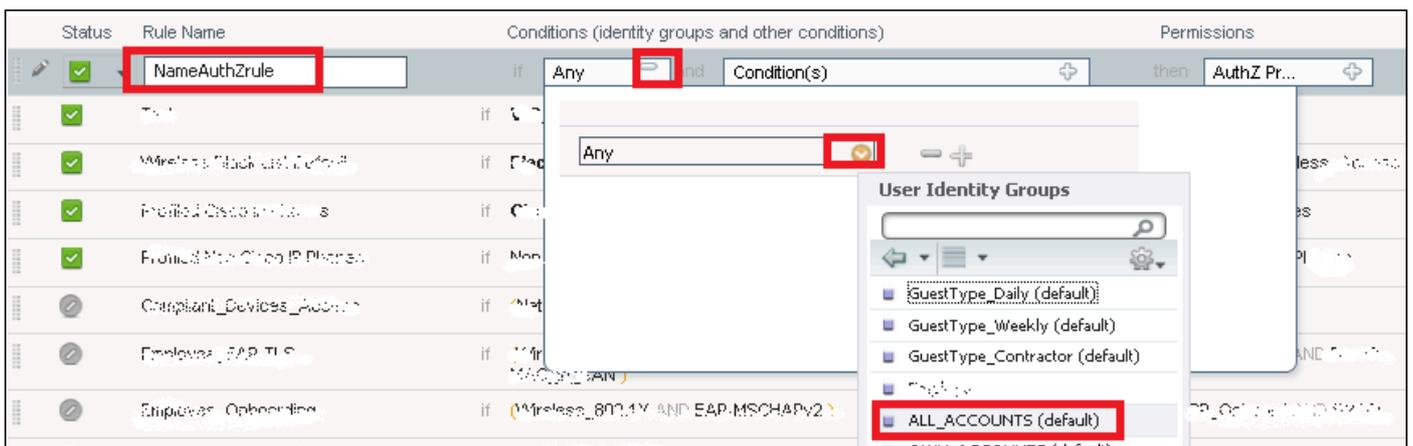
After that choose other conditions that make the authorization process to fall into this rule. In this example the authorization process hits this rule if it uses 802.1x Wireless and it is called station ID ends with *ise-ssid*.
