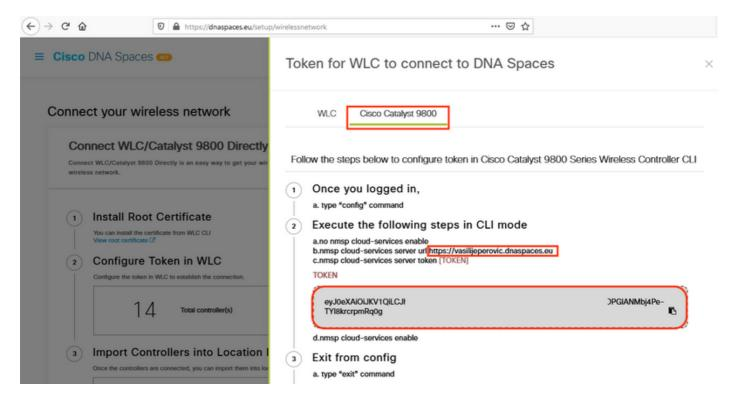
In the WLC web interface, navigate to **Configuration** > **Services** > **Cloud Services** > **DNA Spaces**. Paste URL and Authentication Token. If HTTP proxy is being used, specify its IP address and port.
