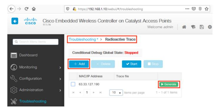
Select **Generate logs** for the last 10 minutes and click Apply. Enabling Internal Logs can generate large amounts of data that might be hard to analyze:
