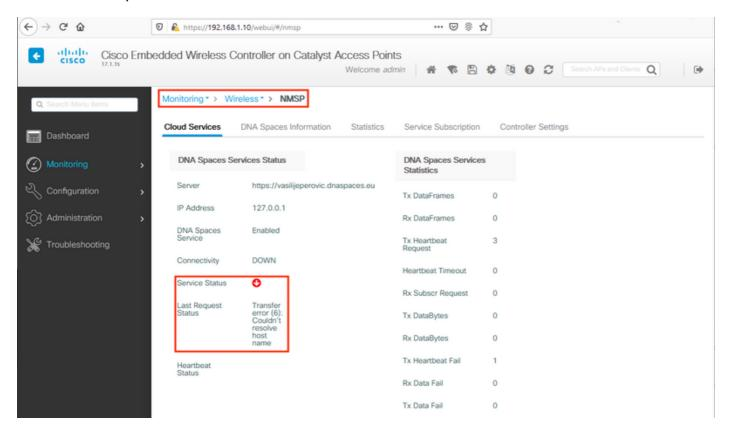
Certificate not being installed or NTP not being configured both result with the error message saying: "Transfer error (60): SSL peer certificate or SSH remote key was not OK":
