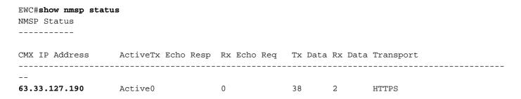
The EWC in this test setup is connecting to 63.33.127.190. Copy this IP address and navigate to **Troubleshooting** > **Radioactive Trace**. Click Add, paste the IP address and click Generate:
