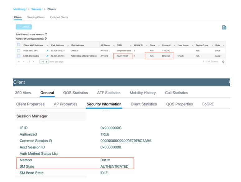
vk-9800-1#show wireless client summary Number of Clients: 2 MAC Address AP Name Type ID State Protocol Method 503e.aab7.0ff4 AP1815 WLAN 3 Run 11n(2.4) None b496.9126.dd6c AP1810 RLAN 1 Run Ethernet Dot1x Local Number of Excluded Clients: 0
