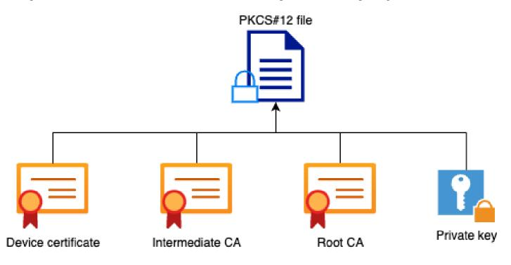
The first thing that you would need to do is to combine all intermediate CAs and the Root CA file into a single file. Copy and paste the contents together (save the file in .pem format) :
