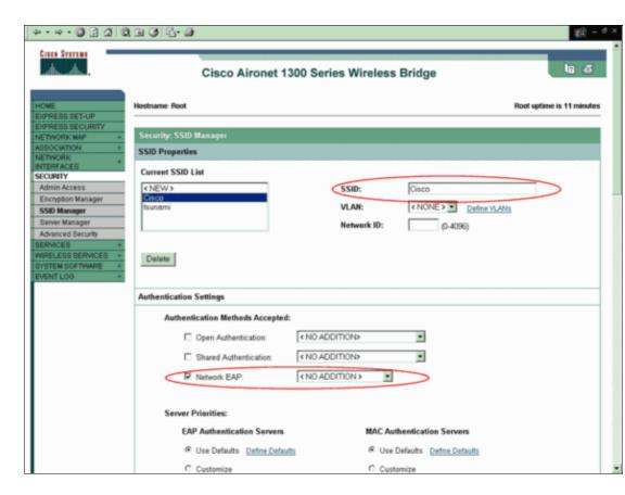
**Note:** In Cisco IOS Software Release 12.3(4)JA and later, you configure SSIDs globally and then apply them to a specific radio interface. Refer to the *Creating an SSID Globally* section of the document Configuring Multiple SSIDs in order to configure SSIDs globally. Also, in Cisco IOS Software Release 12.3(7)JA, there is no default SSID.
