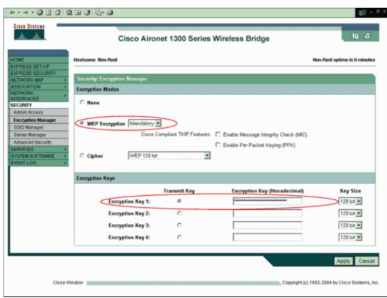
c. In the Encryption Keys area, choose **128 bit** as the Key Size and enter the Encryption Key.
