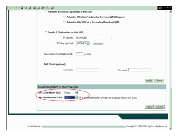
a. From both the Set Guest Mode SSID and the Set Infrastructure SSID drop-down menus, select the SSID that you configured.
