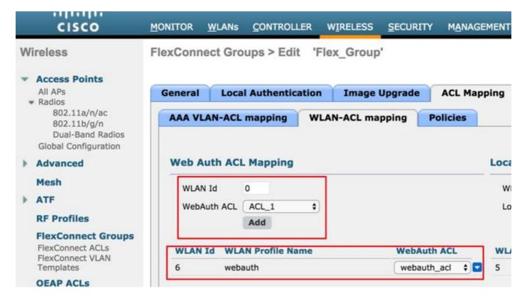
The ACL can be applied at the AP level, navigate to Wireless >AII AP's >AP name >Flexconnect tab > External WebAuthentication ACLs > WLAN ACL as shown in the image.
