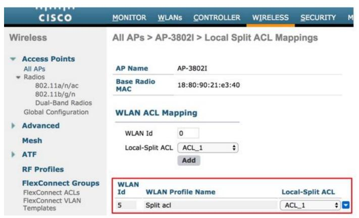
Split Tunneling ACL's cannot locally bridge Multicast/Broadcast traffic. Multicast/Broadcast traffic is switched centrally even if it matches the FlexConnect ACL.
