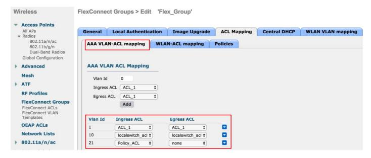
It can also be configured as per the AP level, navigate to **Wireless > All AP's > AP name > Flexconnect tab** and click **VLAN mappings** section. Here, you need to make the VLAN config AP specific first, after which you can specify the AP level VLAN-ACL mapping as shown in the image.
