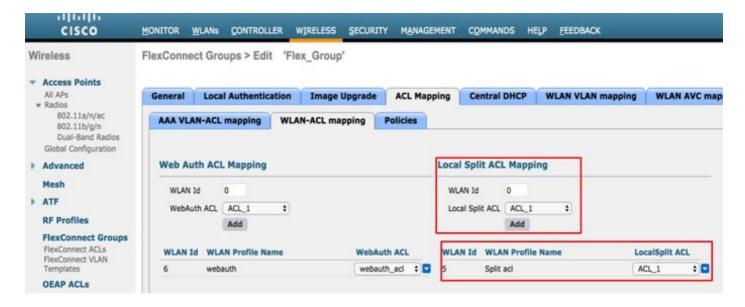
They can also be configured at as per AP level, navigate to **Wireless > All AP's > AP name > Flexconnect tab > Local Split ACLs** and add the name of the flexconnect ACL as shown in the image.
