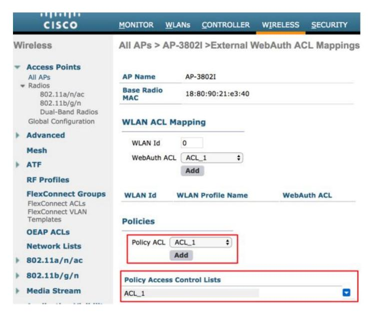
After a successful L2 authentication, when the radius server sends the ACL name in the redirectacl AV pair, this gets applied directly for the client on the AP. When the client moves into **RUN** state, all client traffic is switched locally and the AP stops to apply ACL.
