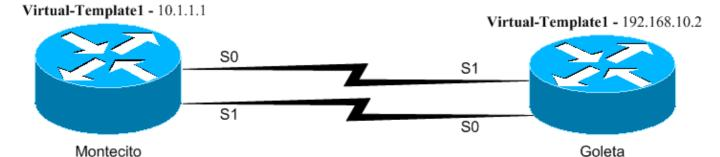
Routers Montecito and Goleta are connected back—to—back through interfaces Serial0 and Serial1. This configuration uses a Virtual—Template on each side, Multilink Point—to—Point Protocol (PPP), and bridges and routes IP and IPX between the routers.
