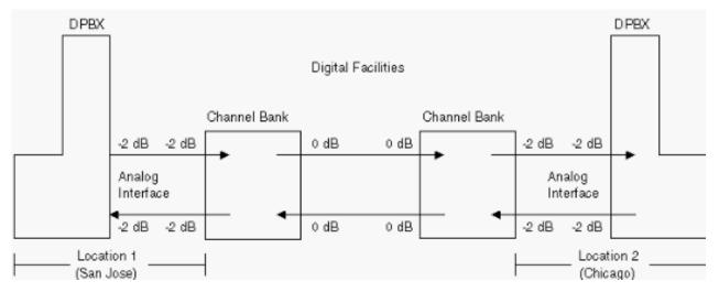
If there is only one CB and it connects to a DPBX through an analog interface, the levels are -2.0 dB transmit and -4.0 receive (see this figure).
