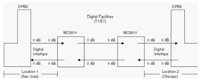
For the majority of Cisco MC3810 implementations, DPBXs are part of the overall customer network. For example, the network topology can look like this:
