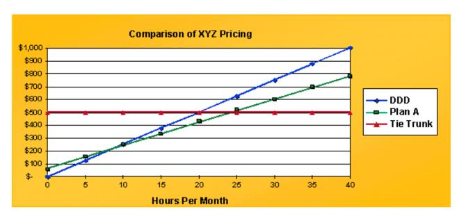
The Tie Trunk, represented by the red line, is a straight line at \$500. DDD is a linear line that starts at 0. To optimize costs, the goal is to stay below the curve. The cross-over points between the different plans occur at 8.57 hours between DDD and Plan A,
