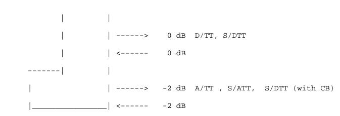
The interfaces and levels expected by DPBXs are listed first in order to help design and implement the Cisco MC3810s with the correct transmit and receive levels. DPBXs with pure digital tie trunks (no analog-to-digital conversions) always receive and transmit at 0 dB (D/TT), as illustrated in the previous figure.
