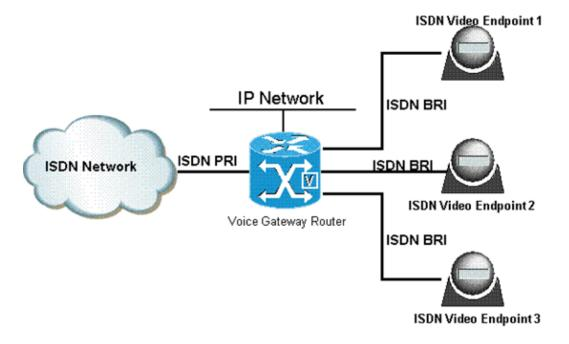
The ISDN PRI to the ISDN network uses E1 interface 0/0/0 with the configuration of 10 B channels. The video endpoints use EM-4BRI-NT/TE BRI interfaces on an EVM-HD-8FXS/DID, slots 2/0/16, 2/0/17, and 2/0/18.
