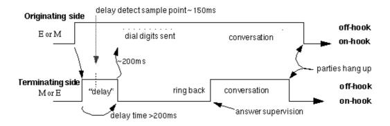
In Cisco 1750, 2600, 2800, 3600, 3800, and VG200 (using an E&M VIC), the default wink delay is 200 ms. See the Verify Delay Dial Signaling Delay sample output for more information on how to verify and modify the Delay Dial signaling parameters.
