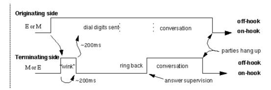
In Cisco 1750, 2600, 2800, 3600, 3800, and VG200 routers (using an E&M Voice Interface Card [VIC]), (with an E&M analog personality module [APM]), the default wink delay is 200 ms. See the Verify Wink Start Signaling Delay output for more information on how to verify and modify the wink delay parameters.
